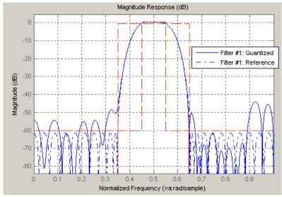
As the figure shows, the filter design constraints are not met. The attenuation is not complete, and there is noise at the edges of the stopbands. You can experiment with different coefficient word lengths if you like. For this example, however, the word length of 12 is sufficient.
