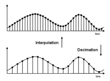
If you start with the top signal, sampled at a frequency Fs, then the bottom signal is sampled at Fs/2 frequency. In this case, the decimation factor, or M, is 2.
